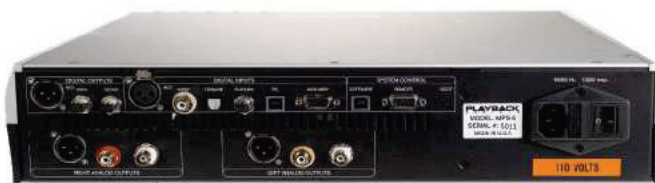
Digital I/O along the top; analog outputs along the bottom.
